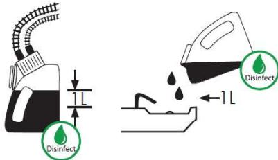
Allow to work for a minimum of one hour or leave overnight. When placing the system back into operation, suction up 2 litres of water.
