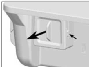
② Press the side lock and remove the CAN dongle.
