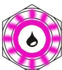
Push-button of the WSU flashes magenta. The WSU stops! The filling process of the supplied water is too slow. Reset the WSU by keeping the button pressed for 8 seconds and restart it by pressing the button briefly. If the magenta flashes continue, call customer service!
