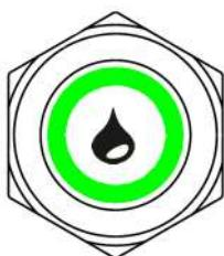
The push-button on the WSU flashes green = start process with start filling. The push-button of the WSU is constantly green = normal operation.
