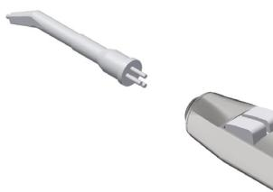
or remove the entire handpiece by pressing the button on the lower part of the handpiece and pulling upwards.
