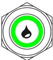
Intensive flushing is activated by a double click on the push-button. The WSU button lights up permanently blue during the phase of double dosage. When the rinsing is activated, the WSU button flashes green-blue. When the rinsing process is finished, the button lights up permanently green. The return to normal operation is indicated on the display.
