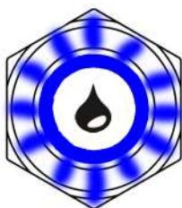
The push-button of the WSU flashes red-blue after a restart of the treatment unit. DK-DOX 150 must be refilled!
