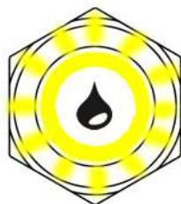
When the push-button of the WSU flashes yellow, DK-DOX 150 must be refilled. You can continue to work without restriction and interruption until the treatment unit is restarted.
