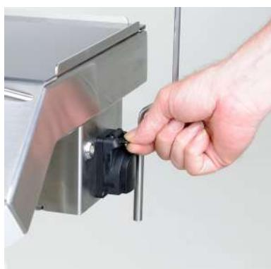
Open the pump cover. Pull the handle upwards.
